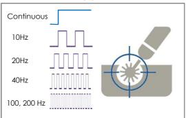
Not only continuous mode but also pulse mode supports for more precise control as similar with CO<sub>2</sub> laser equipment
